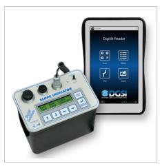
DigiPro2 supports the Digitilt DataMate and the Digitilt AT Reader.
